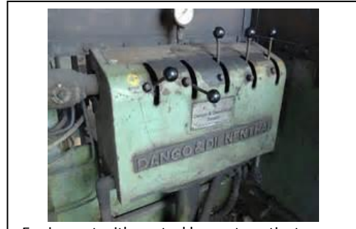
Equipment with control levers to activate mechanical parts must also be tested to verify machinery is inoperable.
