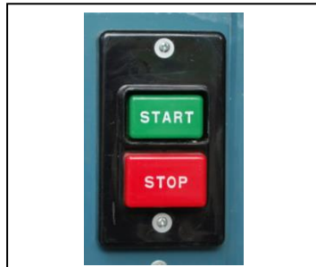
Locate and test the correct start button or switch to verify equipment will not activate.
